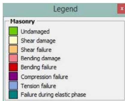
Figure 4. Wall's deformation legend.
